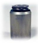
Straight wall: The straight wall punch as it's name suggests has a straight outer walls for use in close quarters where standard punches will not work, and generate a perfectly clean hole in the material being diecut. Keep in mind there is no support bevel on this punch which can make it fragile.
