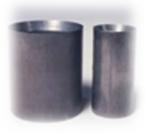
Cup Style: When diecutting these punches the stock is forced into the cup and the compression acts as its own ejector. Cups are generally used for cutting extremely small holes where ejection of scrap can be a problem
