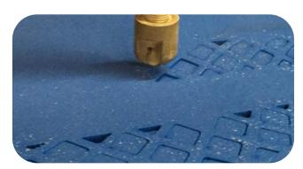
Whether it is a buildup for tooling or a gasket for sealing water-jet cut components are a nice touch to your tooling project. Sharples offers water jet cut rubber ejection producing dies with even ejection; hand cut ejection can cause problems when die-cutting and reduce the quality of finished parts. Sharples can provide a uniform cut set of ejection rubber. Sharples stocks numerous types of ejection material that we note on your individual specification requirements.
